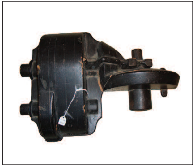
A wooden pattern of the crank case used in the design stage of the Red Rover; a car made in Fulton in 1903. (Photo from Fulton Museum collection.)
